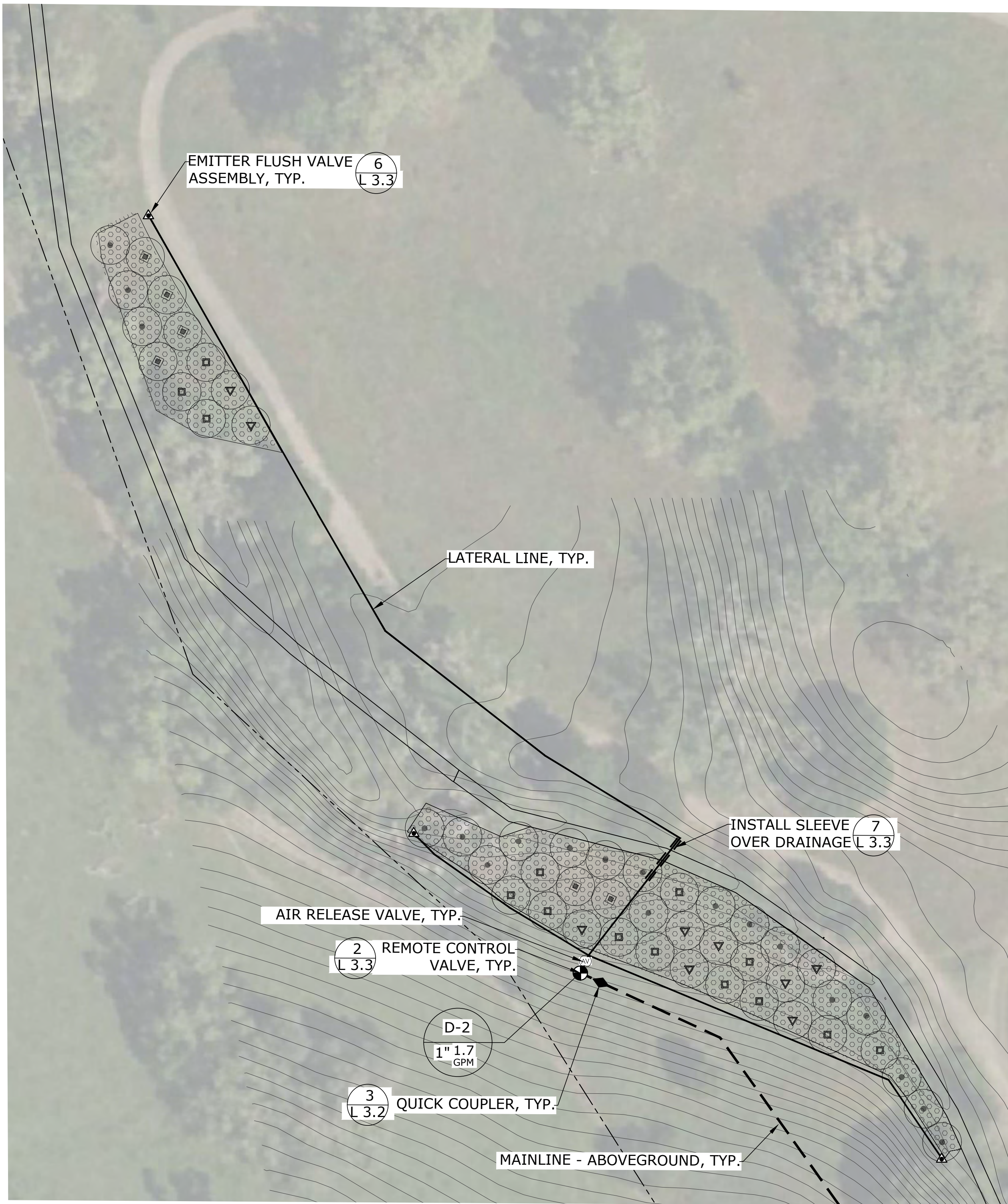
2 IRRIGATION PLAN - MIDDLE AND LOWER FIDDLENECK DRAINAGE SCALE: 1"=30'
