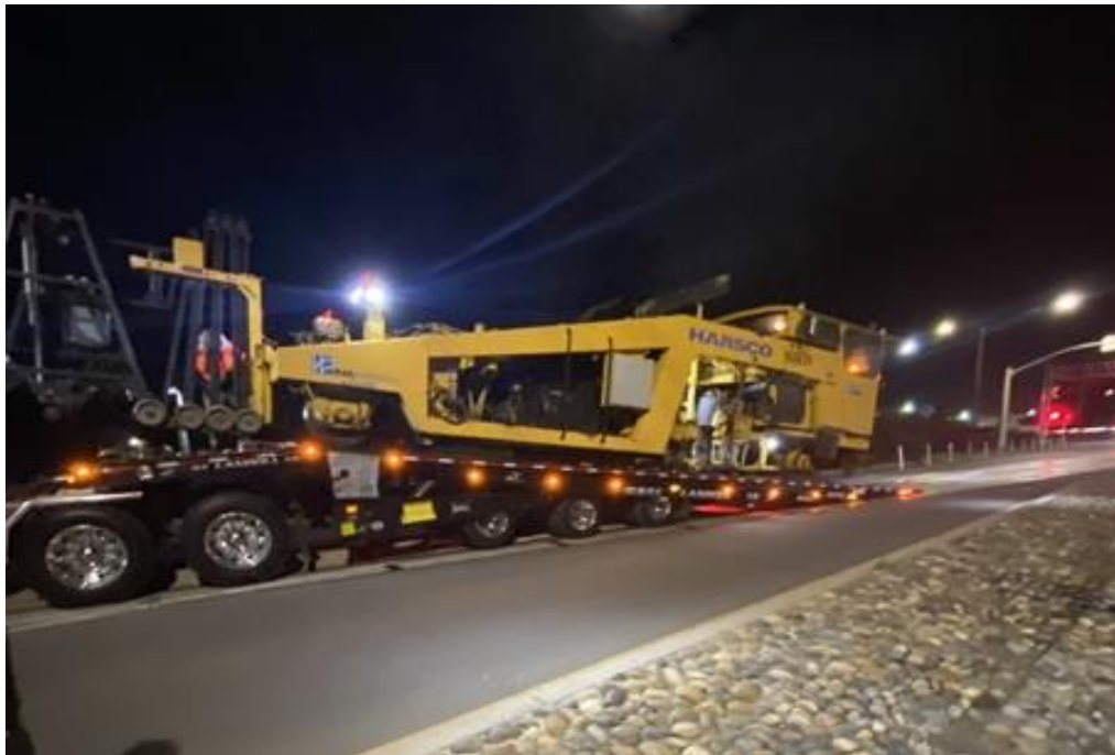
Surfacing equipment (Harsco 6700 Tamper) arriving on site
