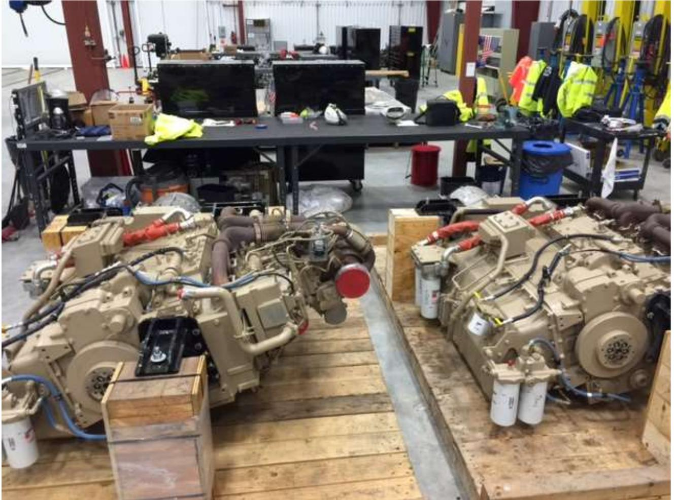
Engines staged for weekly replacement. Six out of 14 cars have had their engines replaced with re-worked ones with new crankshafts and other improvements. Field testing is ongoing and no issues have arisen on the newly replaced engines.
