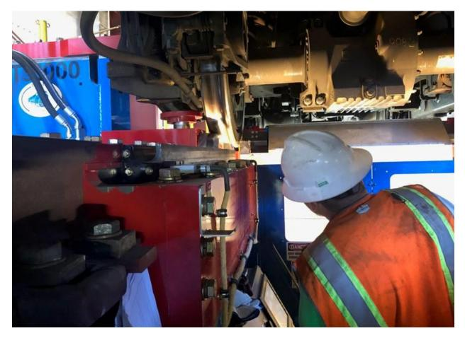
SMART's wheel truing machine has been installed and begun reprofiling wheels that are worn or have flat spots.
