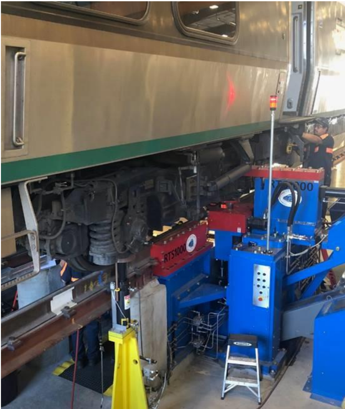
SMART's wheel truing machine is actively truing wheels.
